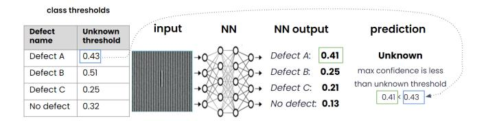
The manual classification augments the existing labelled data and is then used to retrain the Machine Learning model. This way of working avoids the time consuming process of collecting new data for the unseen defects.
