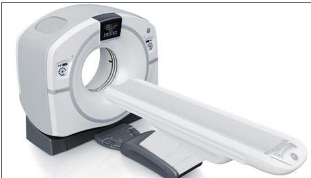
The new GE EVO model replaces the hospital's 16-slice scanner, which has been in use since 2004. Computed tomography uses a combination of X-ray and computer technology to generate three-dimensional views inside the body – including organs, blood vessels, bones and spine. The more image “slices” generated, the faster the scan and the more detailed the 3D rendering.
